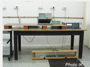
Fig. 2 EMC immunity measurement stand at IK premises in Warsaw
