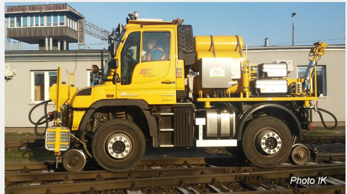
Fig. 2 Road – rail vehicle UniRoller-S intended for rescue and rerailling operations
