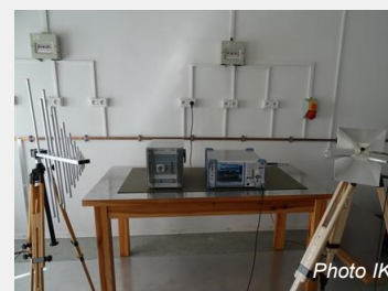
Fig. 3 State-of-the-art measurement equipment for EMC tests purchased by the Railway Research Institute
