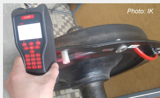
Fig 4. Wheel diameter measurement
