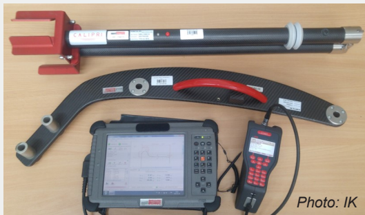
Fig 1. Measuring set for measuring the parameters of wheelsets
