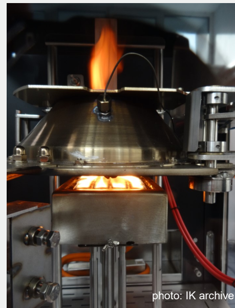
Photo 5. Cone calorimeter for determining the smoke formation and heat release rate for materials exposed to a source of radiant heat (ISO 5660-2:2015) – purchase from IK own resources in 2020
