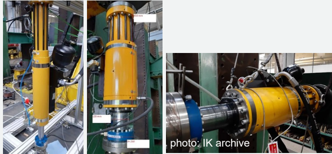
Photo 8. A system of hydropulse actuators from 20 kN to 160 kN for fatigue tests (6 pcs) – purchase under RPMA.01.01.00-14-9845/17-00 Project in 2020
