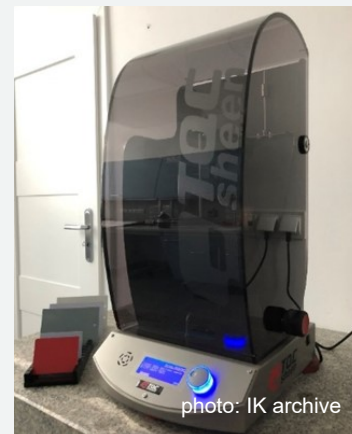
Photo 15. The TQC Sheen TI SP 0500 Pendulum Hardness Tester using the Koning & Persoz pendulum - purchase from IK own resources in 2019
