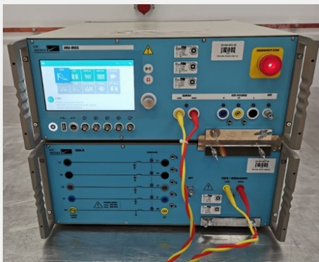
Fig. 1. IMU-MGS generator with an automatic CDN-A-6-32 three-phase network
