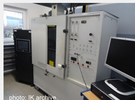
Photo 6. Modernisation of a smoke chamber and apparatus for measuring toxicity based on Fourier Transform Infrared (FTIR) technology together with control and recording systems (according to PN-EN 17084:2019-02 standard) – purchase from IK own resources in 2021
