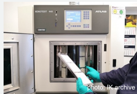
Photo 14. XENOTEST 440 weathering instrument for assessing the resistance to sunlight in the full spectrum of light (UV + VIS + IR) – purchase from IK own resources in 2018
