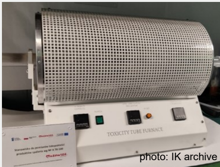
Photo 1. Tube furnace for toxicity measurements – purchase under RPMA.01.01.00-14-9845/17-00 Project in 2019
