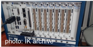
Photo 7. Strain gauge indicator using NI LabView software – purchase under RPMA.01.01.00-14-9845/17-00 Project in 2020
