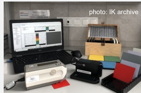
Photo 13. Konica Minolta CM2600D Spectrophotometer and Rhopoint IQ-S Gloss-Meter – purchase from IK own resources in 2018
