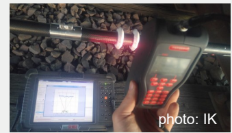
Fig. 4. Measure wheel clearance close-up view
