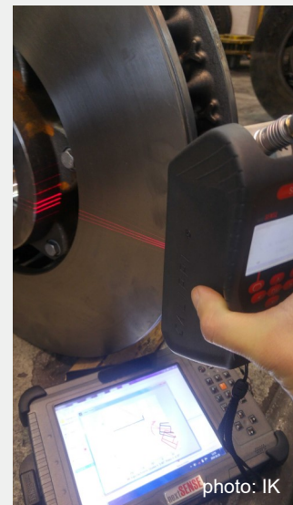
Fig. 5. Measure brake disc wear
