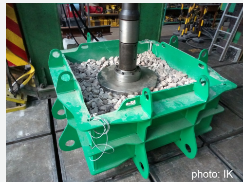
Fig. 3. Test stand for UBM mats
