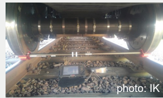
Fig. 3. Measure wheel clearance
