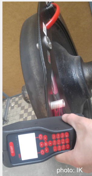
Fig. 2. Measure wheel diameter
