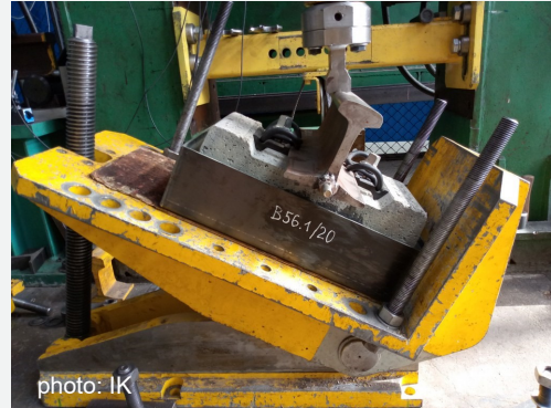
Fig. 2. EBS specimen on the fatigue test stand
