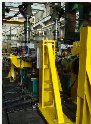
Fig. 1. Tests of vehicle bogie frame, according to PN-EN 13749:2011 standard
