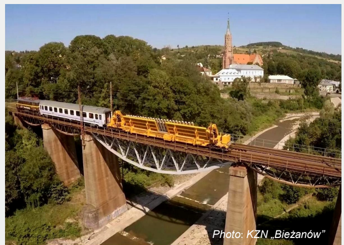
Fig. 6. Dynamic tests of KZN01A type vehicle for transporting railway turnouts on Grybów – Ptaszkowa section
