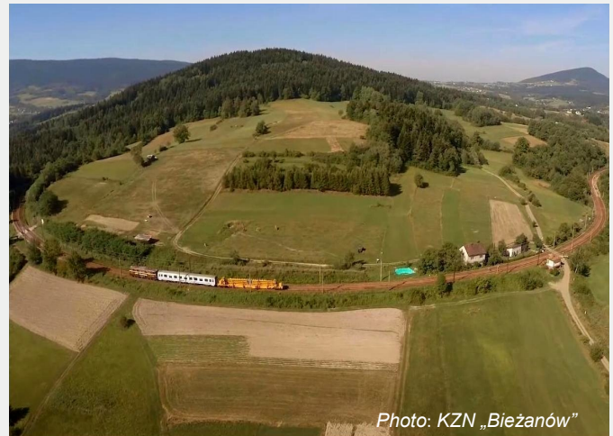
Fig. 5. Dynamic tests of KZN01A type vehicle for transporting railway turnouts on Grybów – Ptaszkowa section
