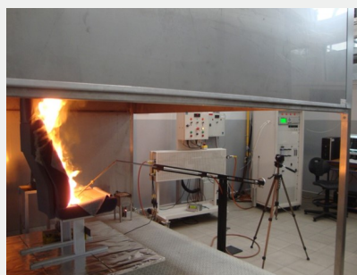
Fig. 1. Tests according to ISO 9705-2 (MARHE, RHR, TSP)
