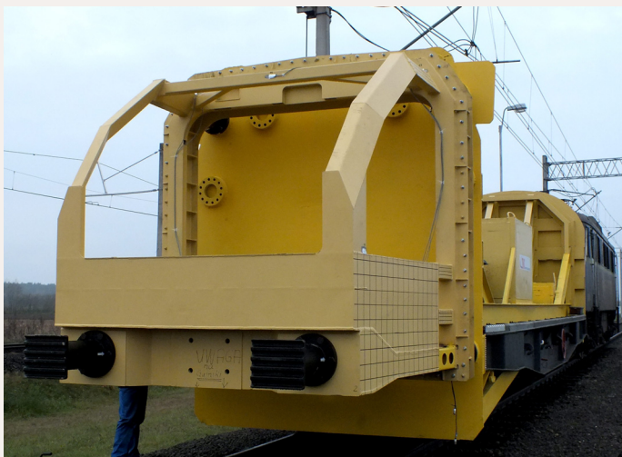
Ram railroad car with mounted driver's cab equipped with side shock absorbers before the test
