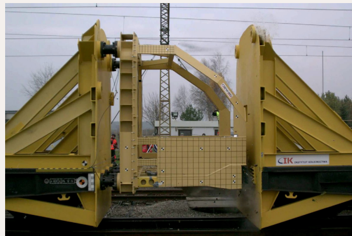
Ram railroad car with mounted driver's cab after the test
