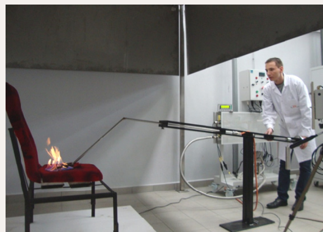
Test stand according to ISO/TR 9705-2 – Reaction to fire tests – Full scale tests or surface products
