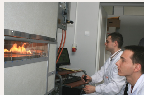
Test stand according to ISO 5660-1 Fire test – Reaction to fire Part1 Rate of heat release
