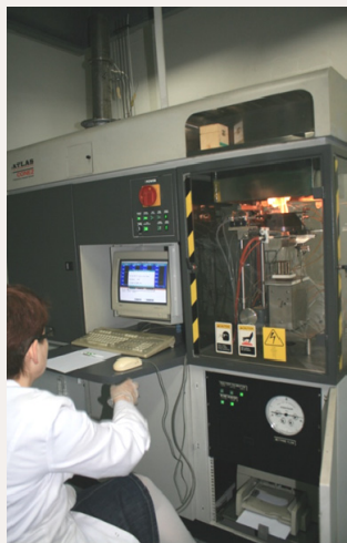
Test stand according to ISO 5660-1 Fire test – Reaction to fire Part1 Rate of heat release
