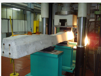
Fig. 2. Stand for examination of sleepers made of long-line prestressed concrete and draw gears on LFV +2500 kN /-4000 kN testing machine
