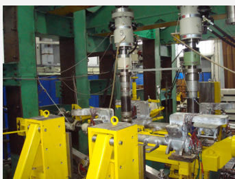
Fig. 1. Stand for examination of bogie frames and oversized objects
