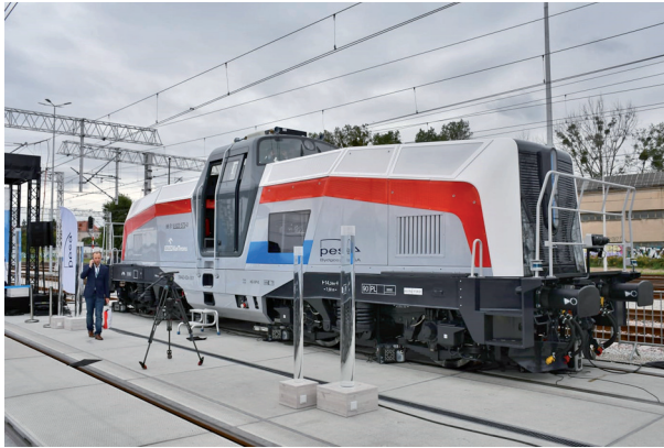
Figure 5.1.9. PESA SM42Dn hydrogen-powered locomotive [44]
