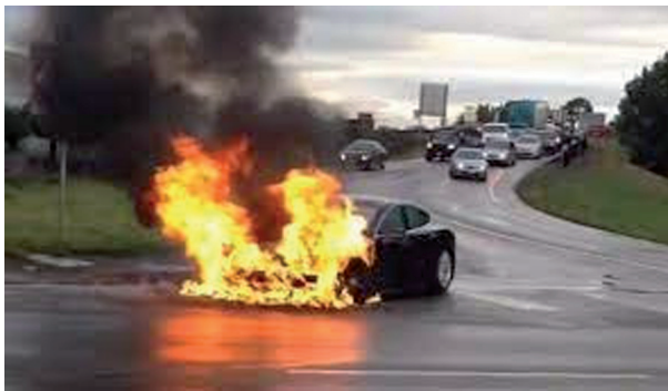
Figure 5.1.4. Lithium battery fire in a Tesla car [49]
